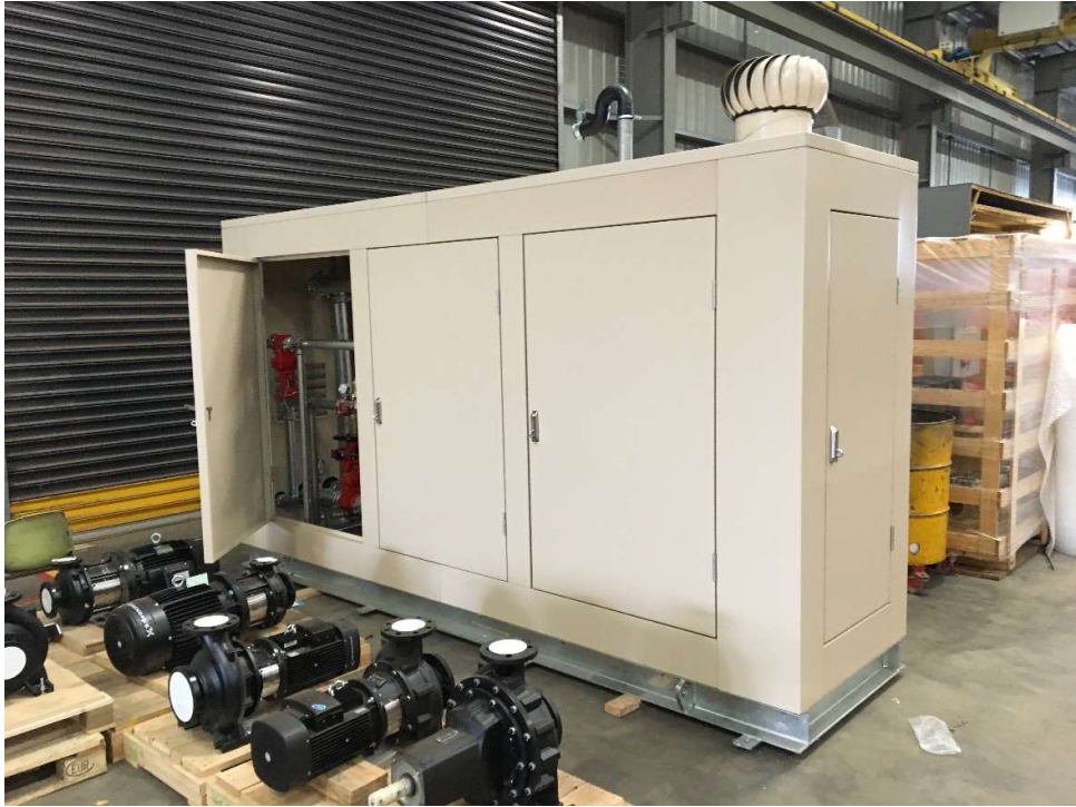
Single diesel enclosure unit
